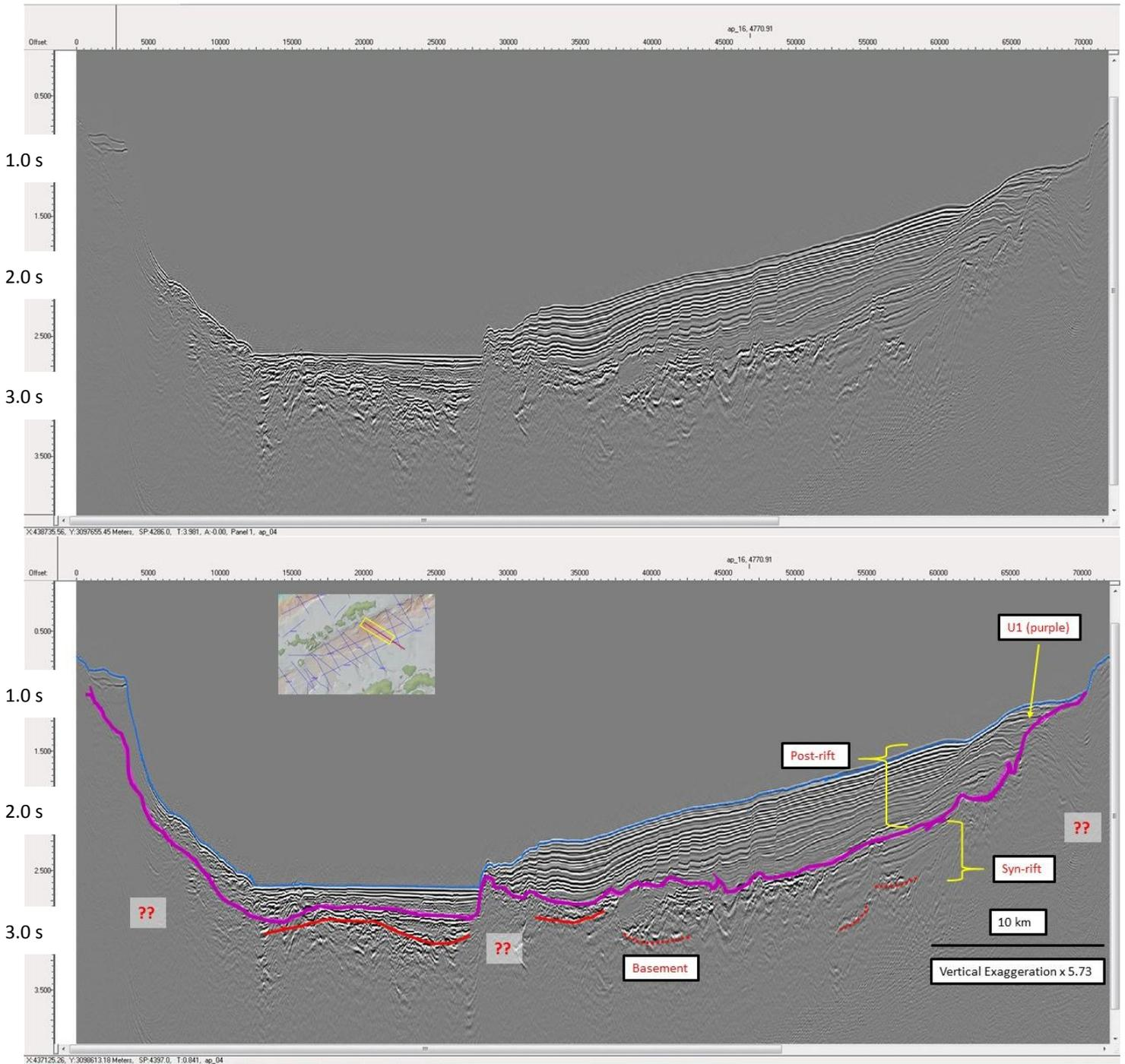
Figure 24. Sedimentary sequences interpretation for the line AP-04. The thick purple line represents the unconformity U1. The solid red lines are interpretations of the basement, while the red dotted lines are interpretations of possible segments of the basement. The interrogations in red represent the areas where the basement could not be observed.
