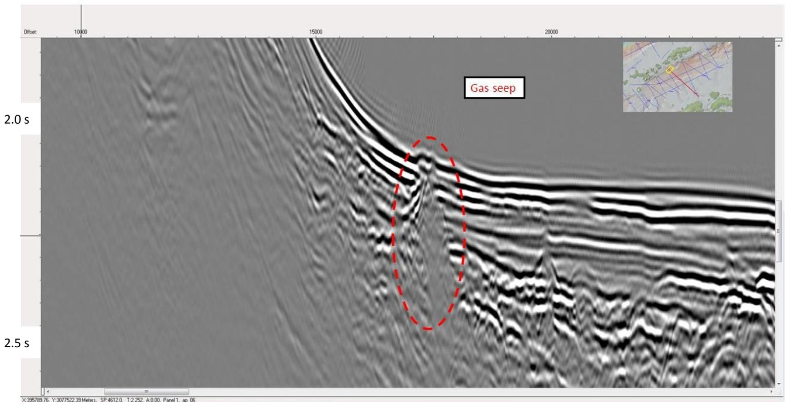
Figure 29. Possible gas seep observed at the continental slope base at the South Shetland Islands margin, identified by the red dotted circle. Seismic profile AP-06.
