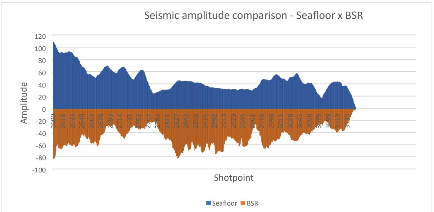
Figure 28. Comparison of seismic amplitudes between the seafloor and the BSR observed on seismic profile AP-03.
