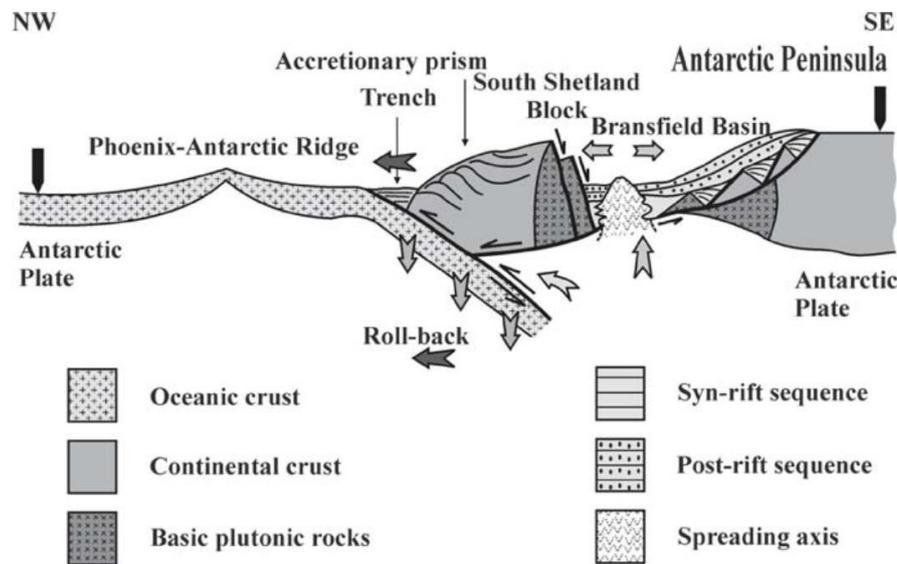
Figure 6. Tectonic sketch interpretation for the tectonic mechanism associated with the Bransfield Strait opening. Taken from Galindo-Zaldívar et al. (2006)
