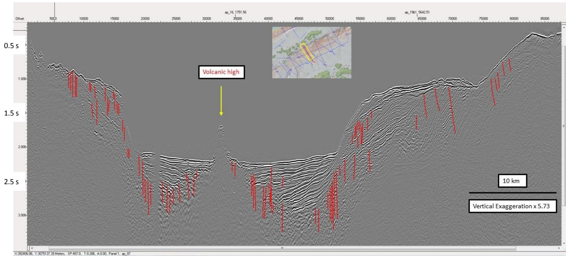
Figure 17. Seismic profile AP-07, identifying volcanic elevations in the central sector of the Central Bransfield Basin.
