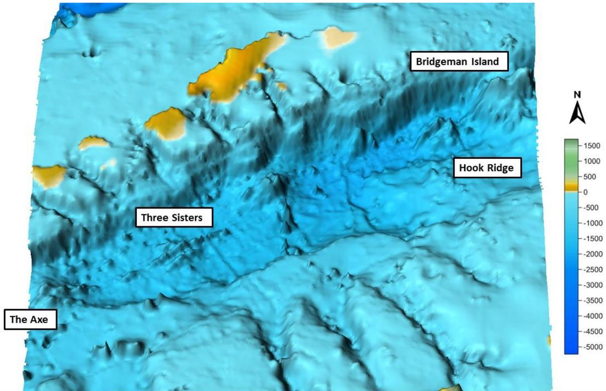
Figure 15. Bathymetry of the Central Bransfield Basin, identifying singular volcanic elevations on the seafloor. Volcanic highs are aligned in a WSW-ENE trend. Data obtained from the ETOPO 1 database.
