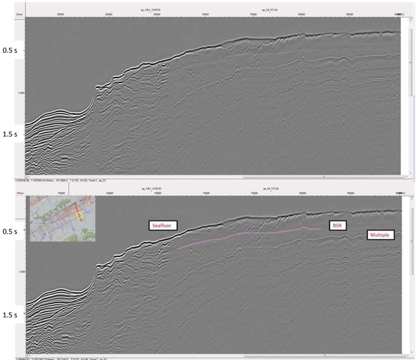
Figure 27. Possible Bottom-Simulating Reflector (BSR) observed at the Antarctic Peninsula margin. Seismic profile AP-03.
