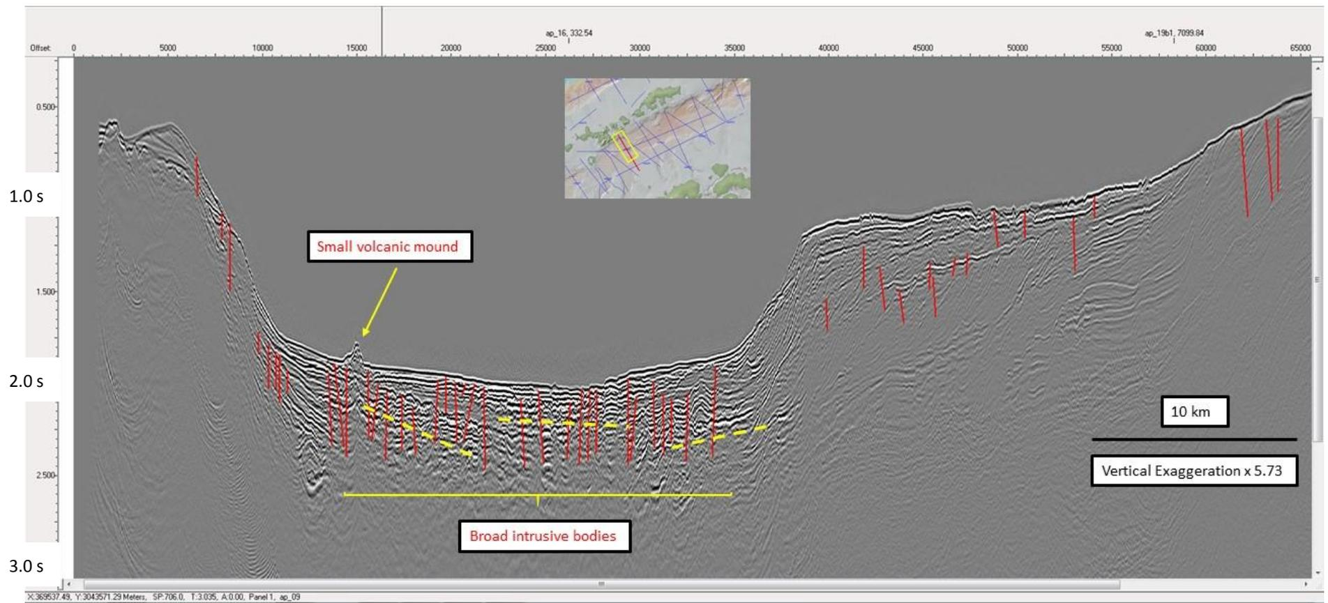
Figure 21. Seismic profile AP-09 identifying a volcanic elevation. Intrusions are interpreted (yellow dotted lines) over a broad area between the sedimentary column.
