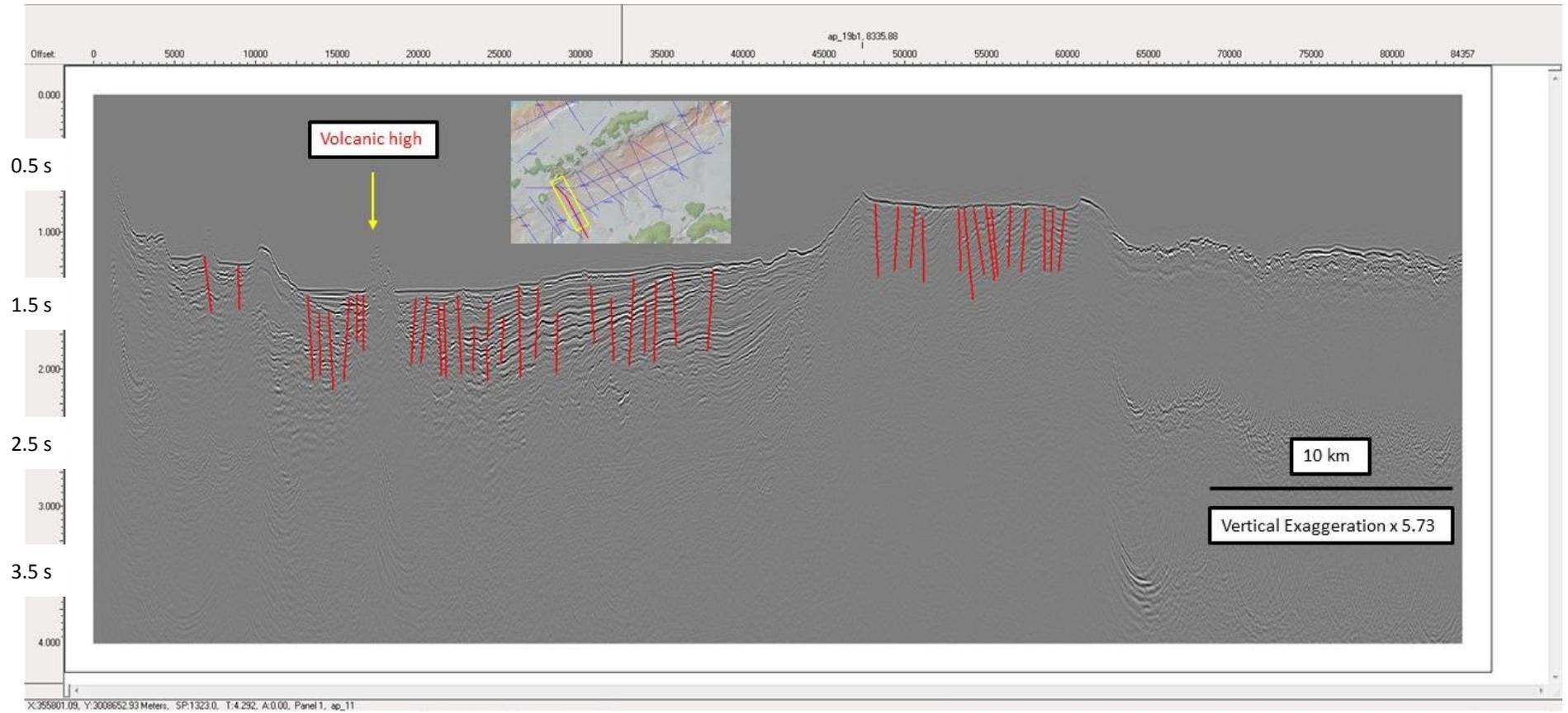
Figure 18. Seismic profile AP-11, identifying volcanic elevations in the western sector of the Central Bransfield Basin.
