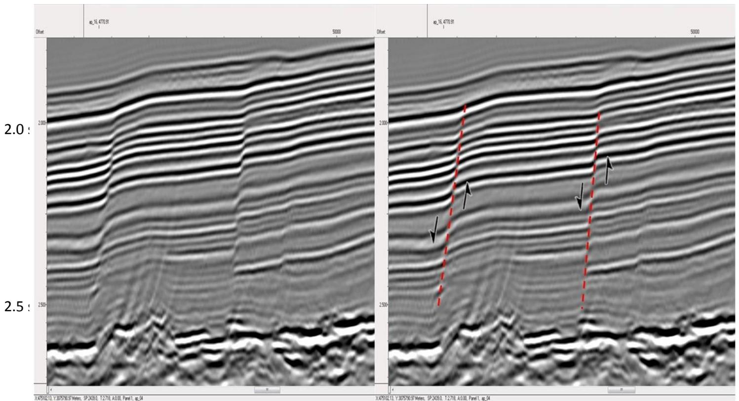
Figure 10. Example of normal faults observed on profile AP-04. The red dotted lines are interpretations of the faults, while the black arrows represent the movement between the faulted blocks.
