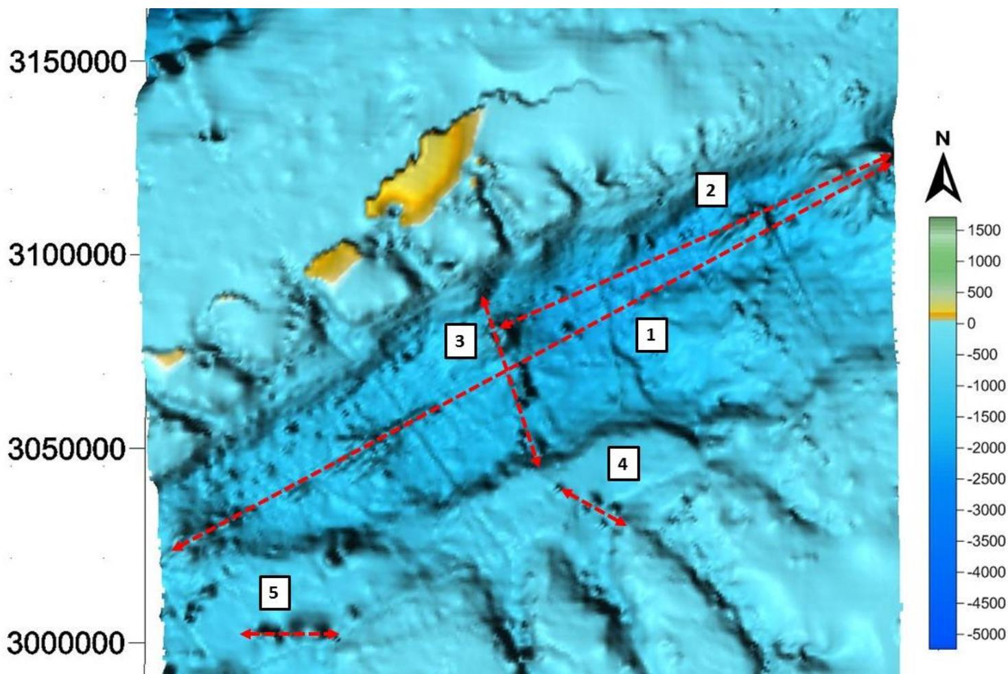
Figure 23. Bathymetry identifying different volcanic mounts orientations observed in the basin, represented by red dotted arrows. Lineation 1 trends WSE-ENE; Lineation 2 trends WSE-ENE; Lineation 3 trends NNW-SSE; Lineation 4 trends NW-SE; Lineation 5 trend E-W.
