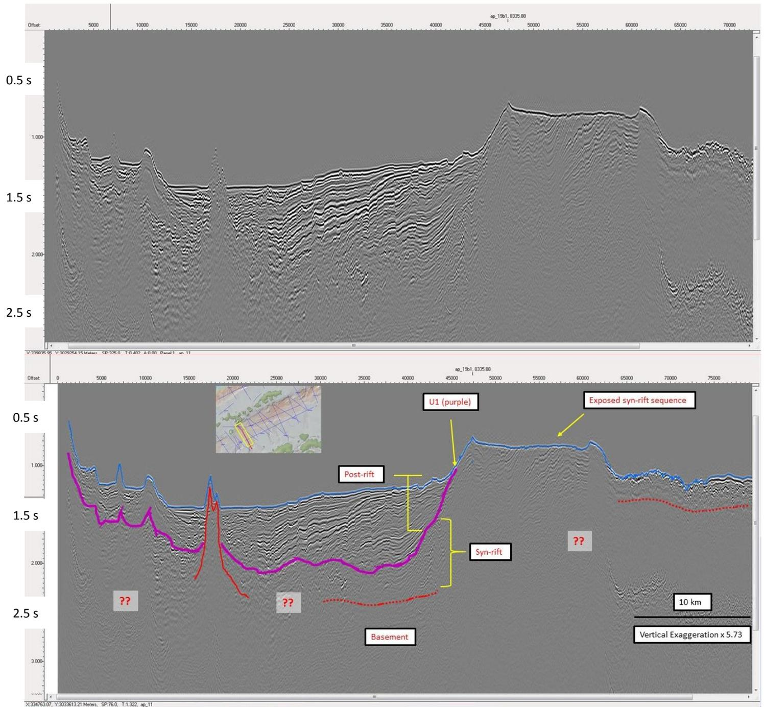
Figure 26. Sedimentary sequences interpretation for the line AP-11. The solid red lines are interpretations of the basement, while the red dotted lines are interpretations of possible segments of the basement. The interrogations in red represent the areas where the basement could not be observed.
