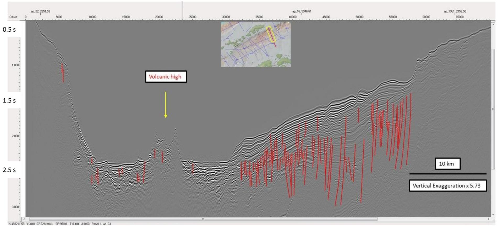
Figure 16. Seismic profile AP-03, identifying volcanic elevations in the eastern sector of the Central Bransfield Basin.
