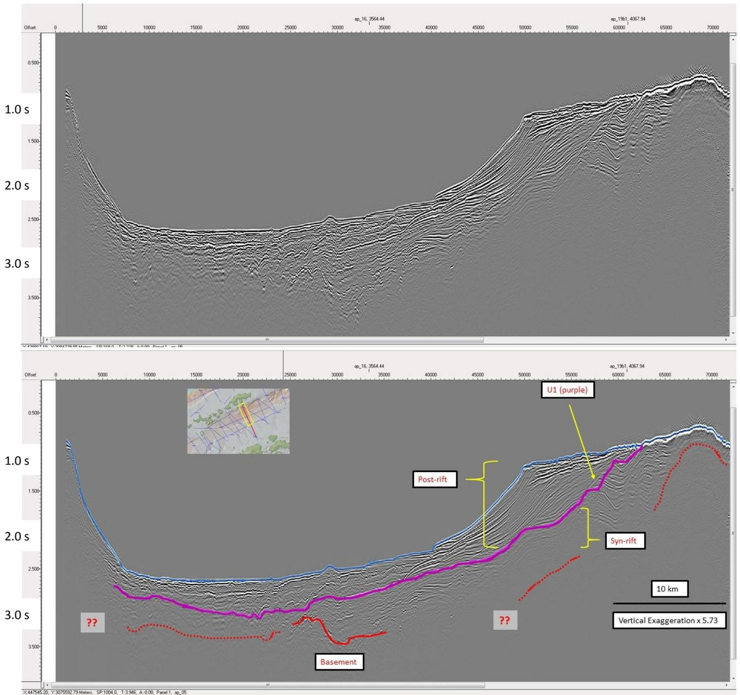
Figure 25. Sedimentary sequences interpretation for the line AP-05. The solid red lines are interpretations of the basement, while the red dotted lines are interpretations of possible segments of the basement. The interrogations in red represent the areas where the basement could not be observed.
