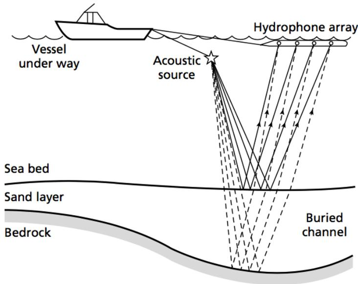
Figure 7. An example of a marine seismic reflection survey. key et al., 2002.
