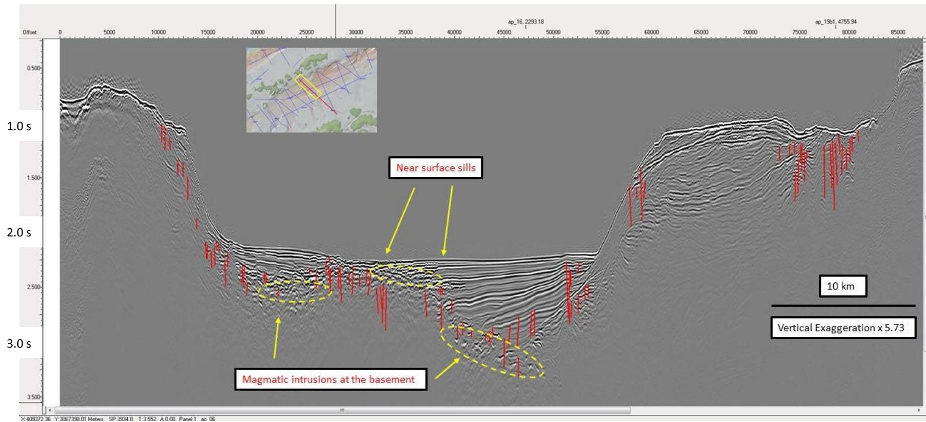
Figure 20. Seismic profile AP-06 which also shows intrusions in the basement. Possible sills are interpreted (yellow dotted circles) over the spreading center.
