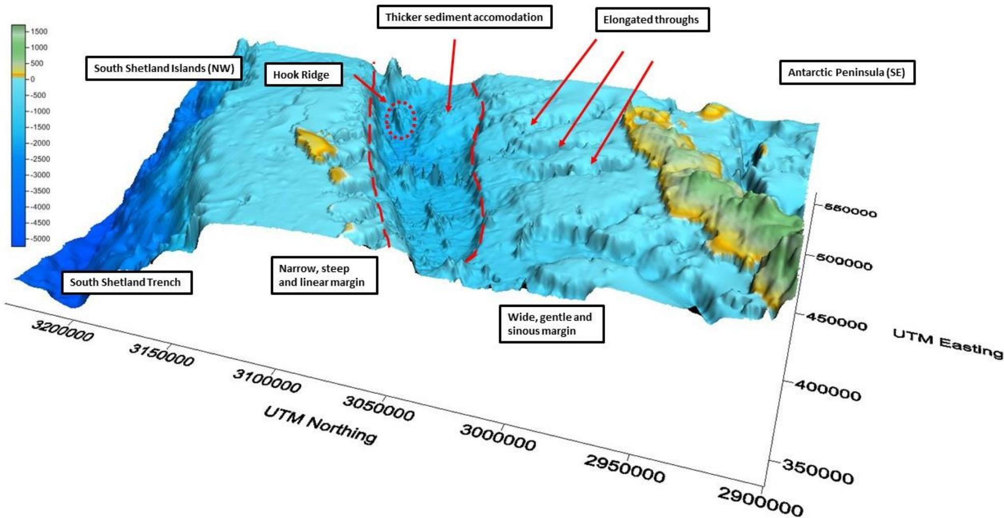
Figure 22. Bathymetry identifying the main morphological features along the Central Bransfield Strait. The red arrows identify important structures, such as elongated throughs and areas with large sediment accommodation. The dotted circle identifies the Hook Ridge volcano at the basin eastern sector, while the dotted lines indicate the continental slope linearity along the basin.
