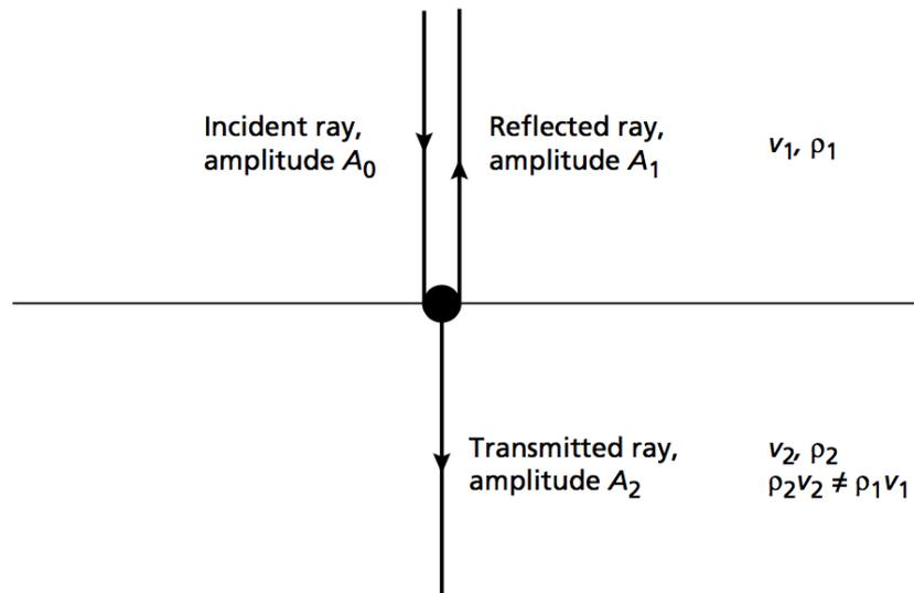
Figure 8. Propagation of rays associated with a normally incident ray on an interface with contrasting acoustic impedance. Kearey et al., 2002.
