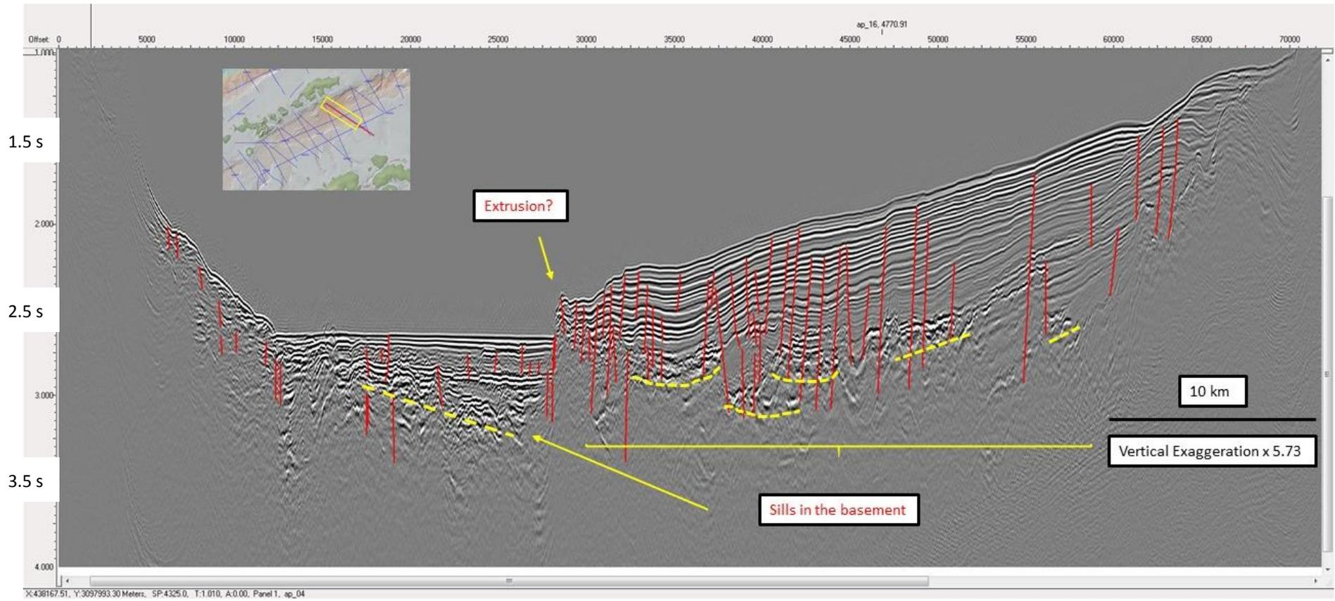
Figure 19. Seismic profile AP-04 showing intrusions in the basement. Some intrusions are interpreted as possible sills (yellow dotted lines), considering their strong lateral signature. A possible extrusive high isolate the sedimentary strata over the basin center.
