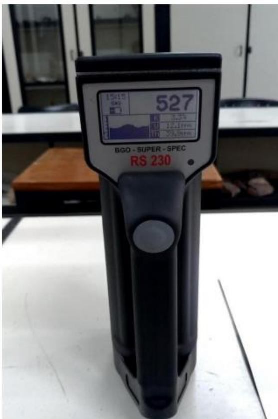
Figura 13: Gamaespectrômetro RS-230 - RadiationSolutions (Nobre, 2019)
